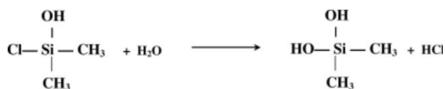
Scheme 2 The hydrolysis step during silane crosslinking.
